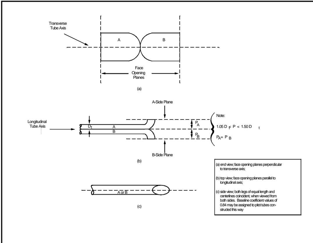
Figure 2-2. Properly Constructed Type S Pitot Tube.
