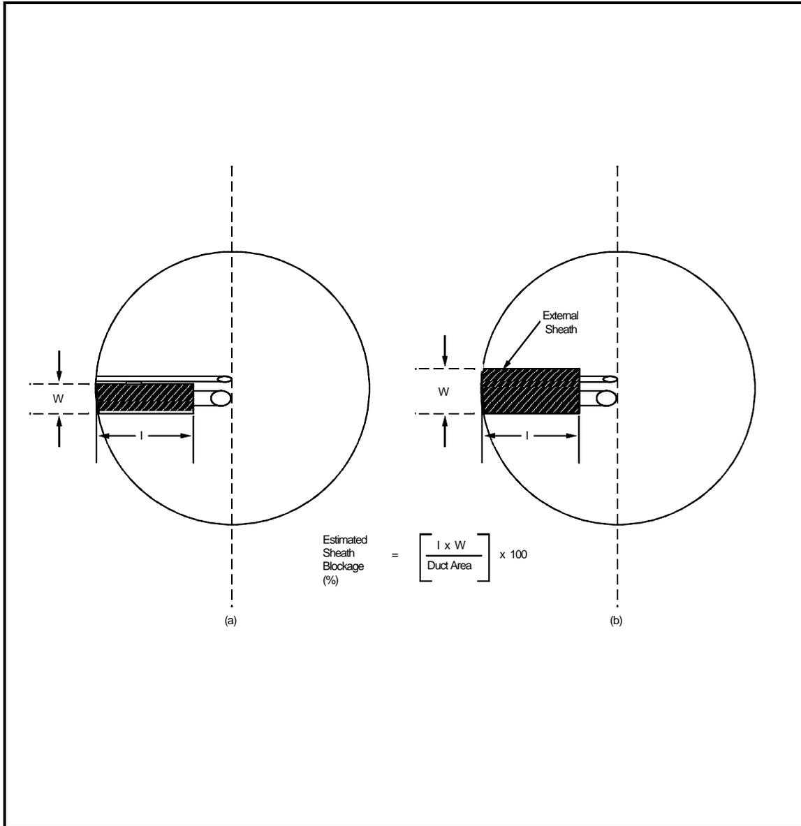
Figure 2-10. Projected-area models for typical pitot tube assemblies
