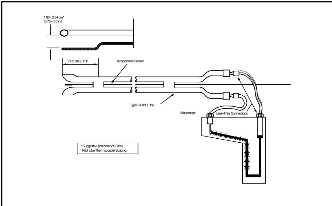
Figure 2-1. Type S Pitot Tube Manometer Assembly.
